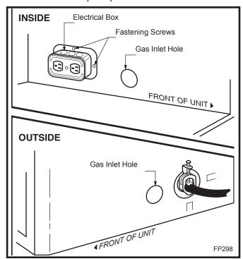
Fig. 8 Junction box (EB-1) hook-up.
